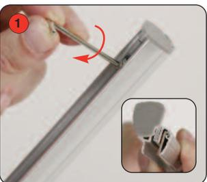
1 Using the Allen key supplied with the user instructions, loosen the top rail screws. Rotate the rail end cap to expose the steel flat bar.
