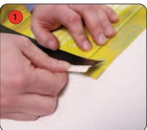
1 Align and adhere the graphic squarely to the slider strip. (attach to front face of graphic)
